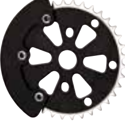
SS-234CNC-166 CNC & chainwheel protector for one piece crank. Teeth: 36, 38T.
